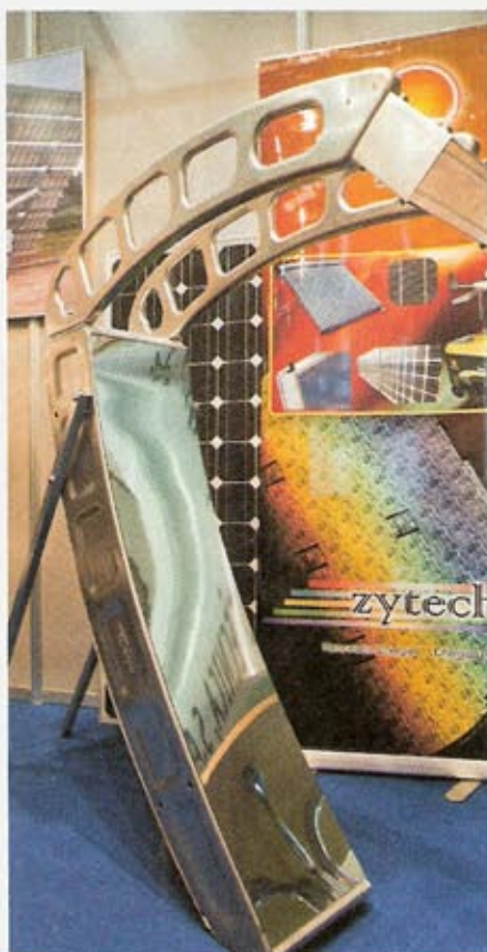
Low CPV: The ZT-2000 C concentrator system (pictured here is a prototype at the Genera trade fair) has mirrors, which concentrate the light by a factor of five.
